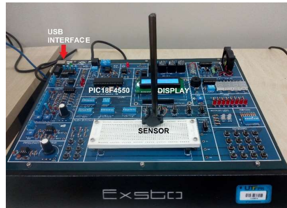
Figure 2. Development kit used by the students in laboratory classes.
