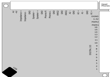
Figure #1: Mobile Studio Desktop™ Software and Hardware Pin Layout
