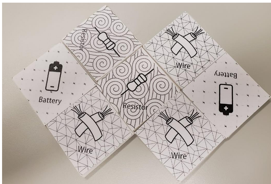
Figure 6. A circuit using two battery and two resistor AR markers for construction.
